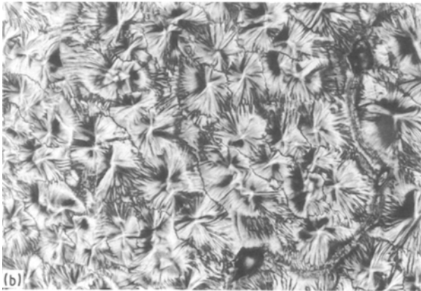
Figure 13 Optical photomicrographs of a-Se annealed under (a) isothermal and (b) non-isothermal conditions.
